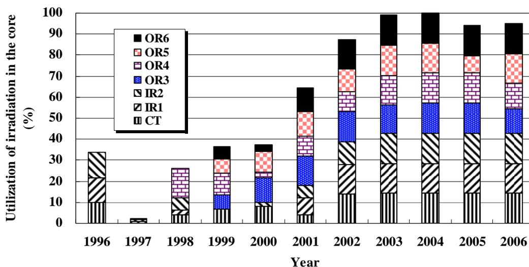
FIG. 2. The status of utilization of the irradiation holes in the core
